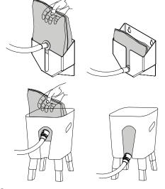
3 ATTACH HOSE TO PUMP: SECURE BY ROTATING TURN KEY CLAMP ON HOSE CLOCKWISE TO TIGHTEN CLAMP AROUND HOSE AND VALVE BODY.
